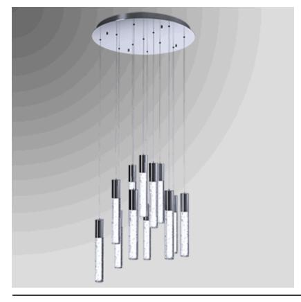
10"H 12-Light Chrome Pendant, direct wired, twelve LED 3 watt, 2880 Lumens, CRI 80, 3000K with Bubble Acrylic Diffuser. Cord adjustable to 59" OAH.
